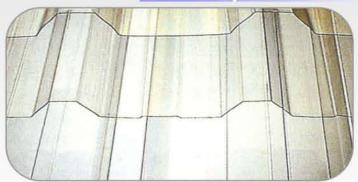
MP-Daylite is rigid polycarbonate transparent roof glazing sheets available in required lengths matching MP-980 or MP-1020 profiles made of out of finest lexan polycarbonate sheets. They offer light transmission between 50%-90% depending on thickness. They also come as one-side embossed thereby increasing the light transmission inside the shed. Their thickness range is between 1 mm to 6mm; however we usually recommend 2mm thickness as the best match with the MP-980 profile type.
